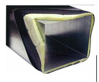
B-10 LAG/QFA-3 is a multi-layered acoustical lagging designed to reduce noise that radiates thru the walls of cluctwork or piping. Cutaway view shows the quilted fiberglass decoupler, the loaded vinyl noise barrier and the outer reinforced foil jacket
