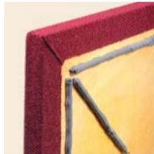
**acouSTIC adhesive installation:** Clean wall surface. Apply  $\frac{1}{4}$ " bead of adhesive around panel perimeter approximately 1"-1 $\frac{1}{2}$ " from panel edge. Apply a  $\frac{1}{4}$ " bead from corner to corner through the center to create an "X." Press panel to surface for 5 seconds. Pull the panel away for approximately 1 minute to allow adhesive to become tacky. Firmly press panel back into position.
